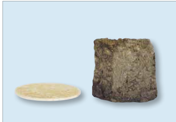
INTERDENS type 36 before and after exposure to fire
